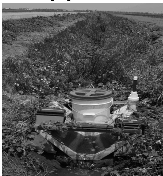
Figure 4. Anderson trial showing vegetated ditch and electronic dosing unit 2008
