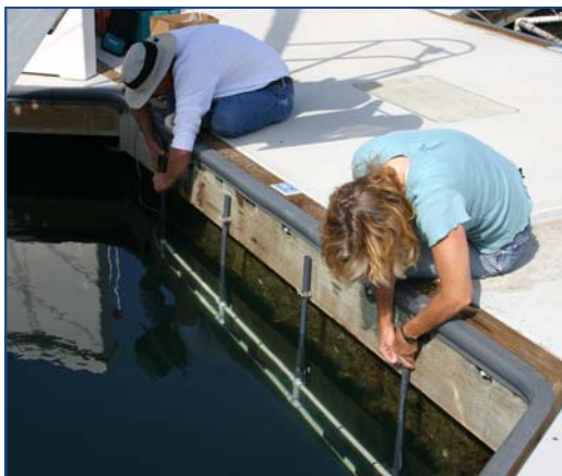
Installing experimental frame and hull coating panels at a San Diego Bay marina
