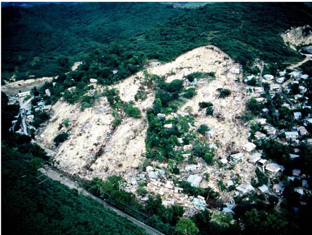
Figure 4. Unplanned community on steep unstable bedrock, Barrio Mameyes, Ponce, southern Puerto Rico. Photo source: R. Jibson, USGS, 1985. Hillslope failure killed 129 people (Jibson, 1989).
