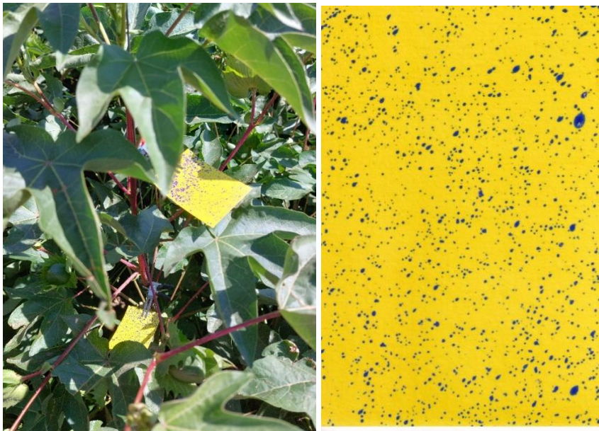
Figure 1. Water-sensitive cards on a cotton plant at the 5 th and 9 th nodes (left). Water sensitive card after an application with spray droplets (right).
