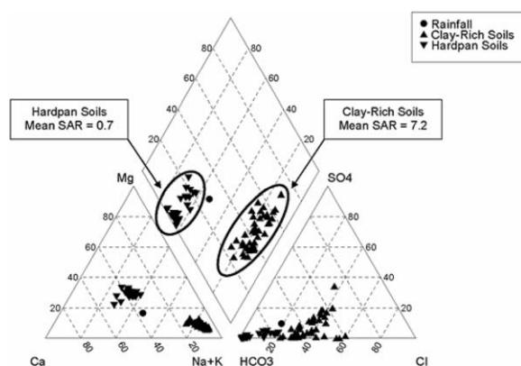
Figure 8. Piper diagram (Piper 1944) indicating that water in the vernal pools on clay-rich and hardpan soils had distinctly different percentage compositions of sodium+potassium, calcium, and magnesium, with vernal pools on clay-rich soils having higher percentage compositions of sodium+potassium and relatively lower percentage compositions of calcium and magnesium.
