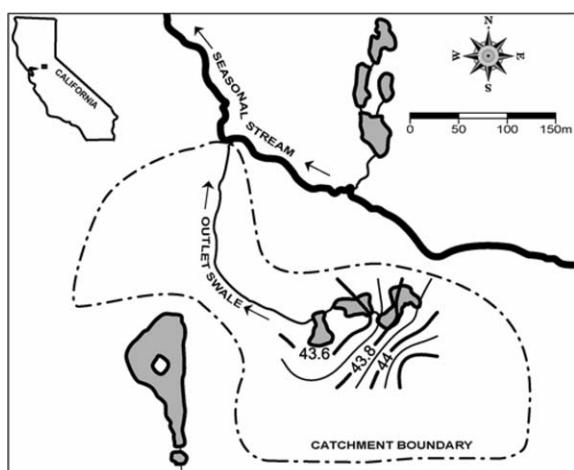
Figure 5. Hydraulic head above the claypan/duripan at the hardpan soil site in meters above mean sea level. Stages in the vernal pools were neglected in generating these contours. Data are from late February 2003, and are similar to data from earlier and later in the wet season.
