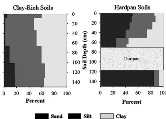
Figure 2. Generic cross-sections of typical pedons for the clay-rich and hardpan soil sites. Data are from pedon IDs 64CA113012 and 79CA067001, respectively, from the U.S. Department of Agriculture Soil Characterization Database (Soil Survey Staff 2006).
