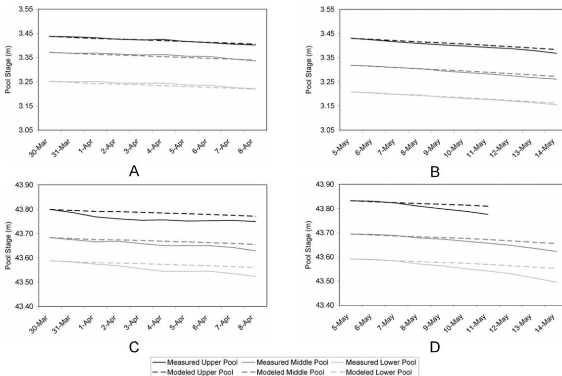
Figure 4. Measured and modeled stages in m above mean sea level during periods of time when there was little to no rainfall for A) vernal pools on clay-rich soils in the middle of the wet season, B) vernal pools on clay-rich soils at the end of the wet season, C) vernal pools on hardpan soils in the middle of the wet season, and D) vernal pools on hardpan soils at the end of the wet season during water year 2003.
