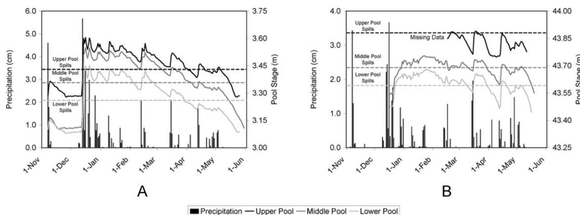
Figure 3. Daily precipitation in cm and stages in m above mean sea level for A) vernal pools on clay-rich soils and B) vernal pools on hardpan soils during water year 2003. Horizontal dashed lines indicate the stages at which surface water flows out of each vernal pool via an outlet swale.
