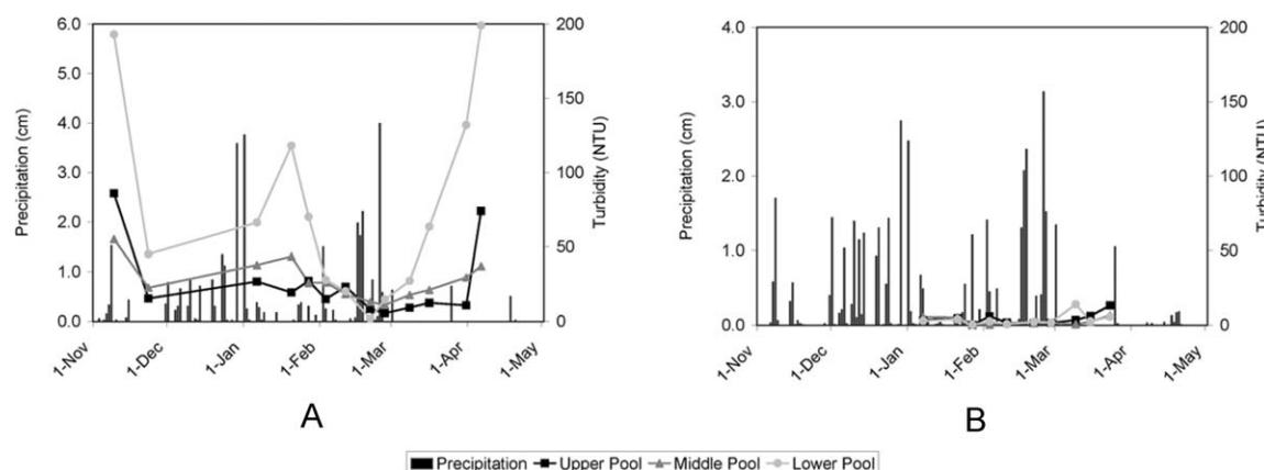
Figure 9. Daily precipitation in cm and turbidity in NTU for A) vernal pools on clay-rich soils and B) vernal pools on hardpan soils during water year 2004.
