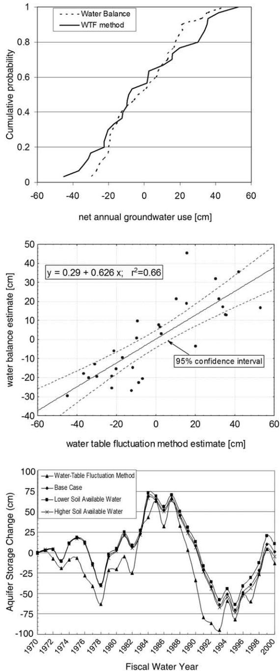
Fig. 7. Annual groundwater storage changes for the study area as computed by the water balance model and the water-table fluctuation method. Top: cumulative probability distribution functions; center: Scatterplot and linear regression; cumulative changes from 1970 to 2000.
