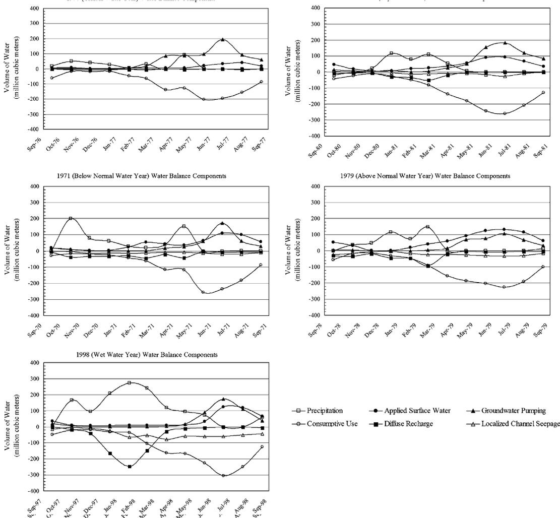
Fig. 6. Monthly water balance components for representative ‘Critical’, ‘Dry’, ‘Below Normal’, ‘Above Normal’, and ‘Wet’ water year types. Fluxes to the land surface are positive, fluxes away from the land surface are negative.
