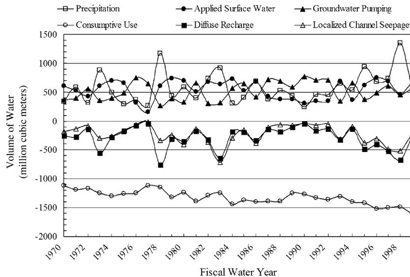
Fig. 5. Annual water balance components of the study area from 1970 to 1999. Fluxes to the land surface are positive, fluxes away from the land surface are negative.
