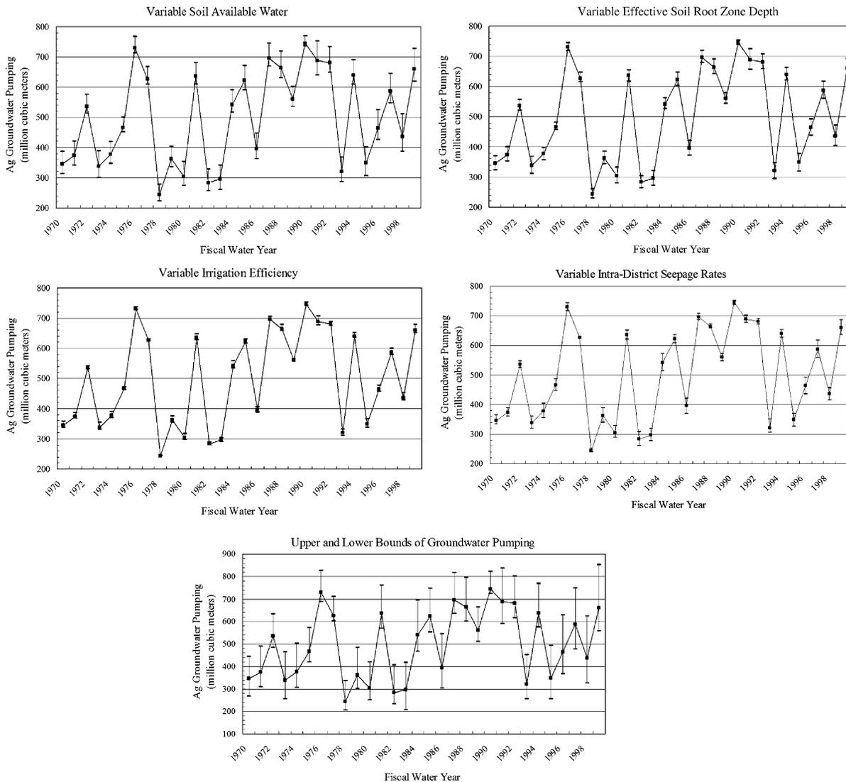
Fig. 8. Estimated annual groundwater pumping for the study area for variable soil available water, effective soil root zone depth, irrigation efficiency, and intra-district seepage rates.
