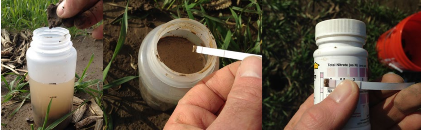
Figure 2. Illustrates several of the steps and materials involved in the soil nitrate quick test method.
