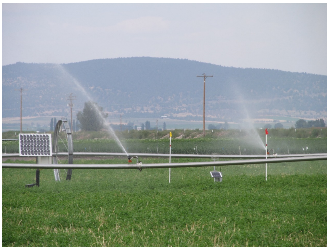
Figure 2. Instruments were installed at IREC alfalfa field to monitor ET. Surface renewal instruments to the left and commercial Tule unit to the right between the flags (Photo: Laurie Askew).
