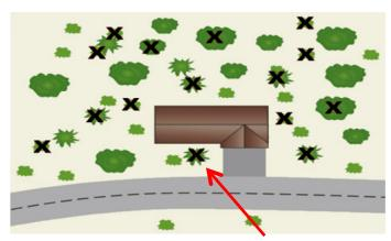
Figure 4. The riskiest locations for planting. The inside corner of the house is where embers 'eddy out' and collect during high wind events. (Photo UCANR Home Landscaping for Fire publication <a href="https://anrcatalog.ucanr.edu/pdf/8228.pdf">https://anrcatalog.ucanr.edu/pdf/8228.pdf</a>)
