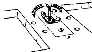
Tighten wing nut to secure the setting. The light will come on when the heat is on. Adjust the temperature for 100°F. for most eggs. Allow the incubator to operate for at least ½ day to stabilize the setting before putting in eggs. (see note above).
