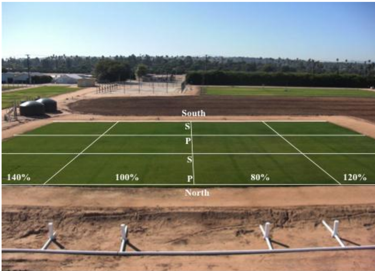
Figure 1. Turfgrass salinity research area in Riverside, CA. Alternating irrigation lines are fed by potable (P) or saline (S) water. Two 5,000-gallon tanks are used to store and deliver saline irrigation water. In the perpendicular direction, the area is divided into four irrigation zones, ranging from replacement of 80 to 140% ET_0 . Two subsurface drain lines bisect each of the irrigation zones with outlets for collection of leachate. Twelve 30-ft x 30-ft plots represent a continuous distribution of saline and potable water at a given irrigation regime.
