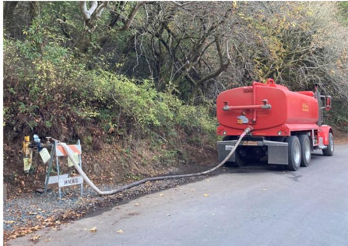
Metered hydrant and truck being filled to haul water to ranches with limited water supplies.
