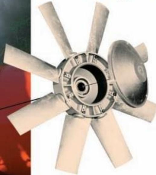
The Pul-blast has a selection of aluminum alloy axial flow fans ranging from 22"-36" diameter. Each fan is fitted to its fan housing to produce optimal performance. 22" and 24" diameter fans have six blades with a fixed pitch. 32" and 36" fans have 8 blades, each with a 3-position variable pitch. 28" diameter fans are available with 6 fixed blades or 8 variable pitch blades.
