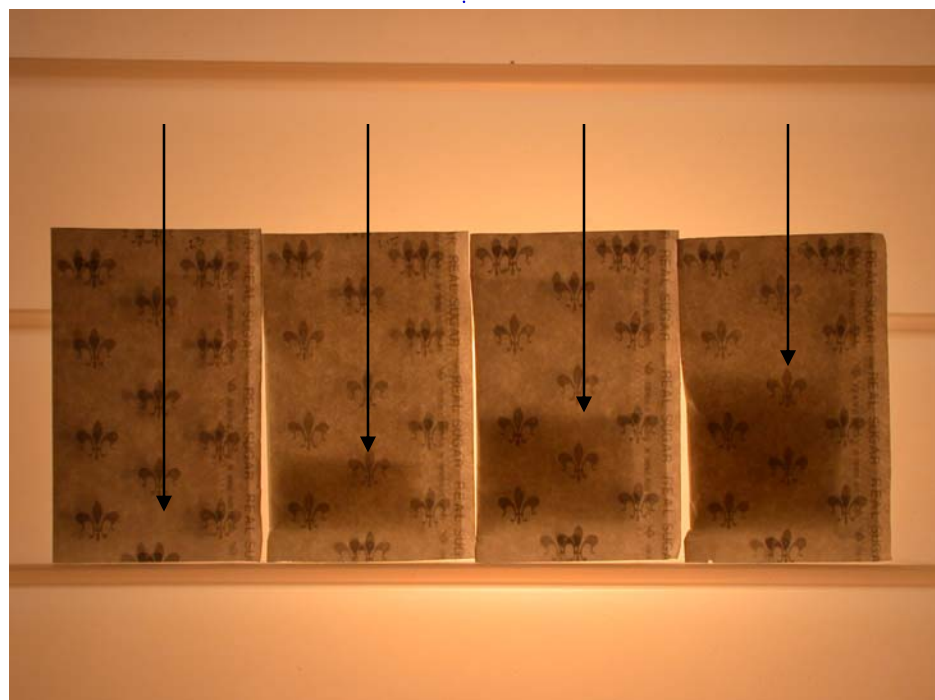
Figure 7. Visual difference in contents of commercial sugar packets. The packet on the far left is empty and the packet on the far right has the expected amount of sugar. Arrows indicate level of sugar in each packet.
