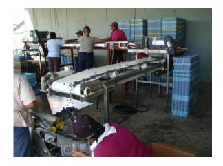
There are various sizes of packaging lines for larger volumes of fruit. Packing lines includes blowers to remove waste, sorting tables to remove the unmarketable fruit and classification screens to eliminate fruit that do not reach the minimum market size. There should be only one layer of fruit on the table for inspection. Packing lines should be cleaned daily with detergent and water, and then spray with a 5% bleach solution (sodium hypochlorite).
