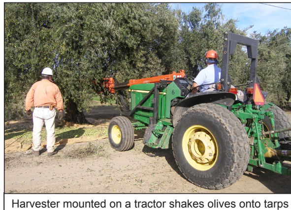
Harvester mounted on a tractor shakes olives onto tarps
