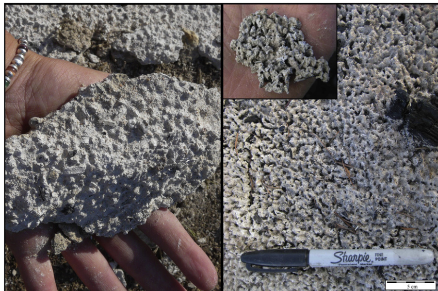
Fig. 8. Left: Crusted ash produced in the laboratory at temperatures >900 °C. Right: Ash crust formed during high severity wildfire in Montana, USA (Balfour et al., in review).
