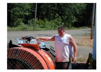
3. Measure the amount of water it takes to fill the sprayer back up to the line observed in 1.
