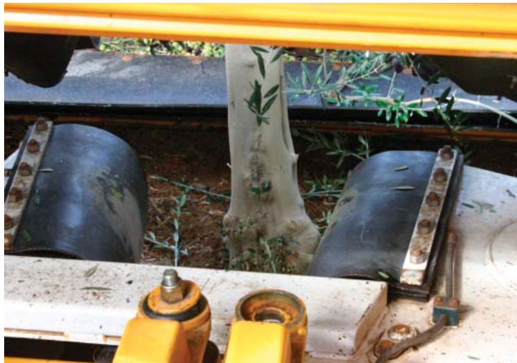
A side-by-side shaker harvester grabs the trunk of an olive tree while the catch-frame moves into place
