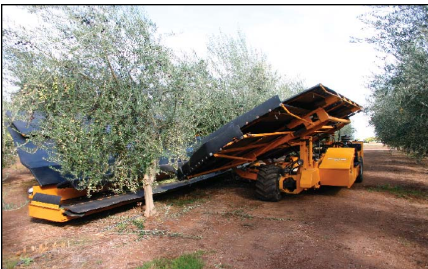
The side-by-side shaker harvester moving into position on an olive tree
