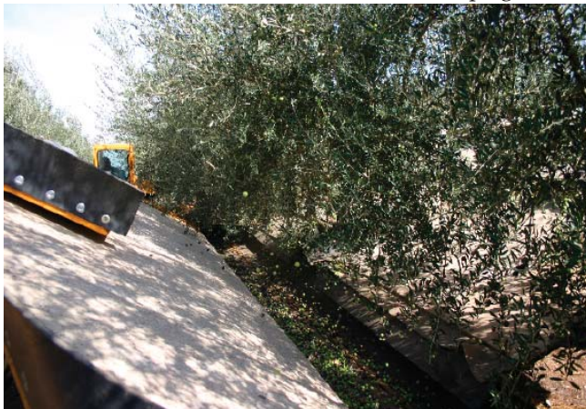
The fruit collects in the valley formed by the shaker and collector and is conveyed to a bin.
