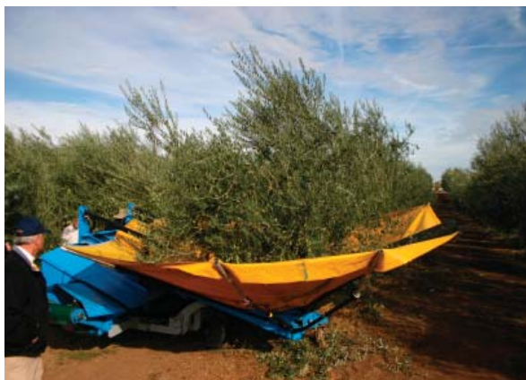
The wrap-around umbrella-type catch frame is one option for collection with a shaker harvester.
