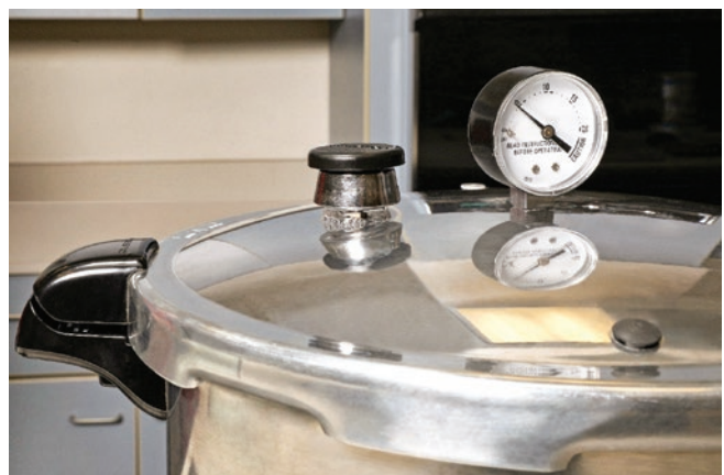
Figure 19. Allow the canner to depressurize normally without assistance.
