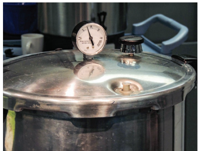
Figure 6. The dial gauge is a delicate instrument and must be tested each year for accuracy. Courtesy of Colorado State University.
