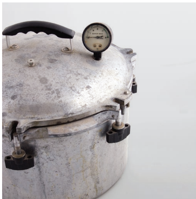
Figure 10. Pressure canner with corrosion and pitting.
