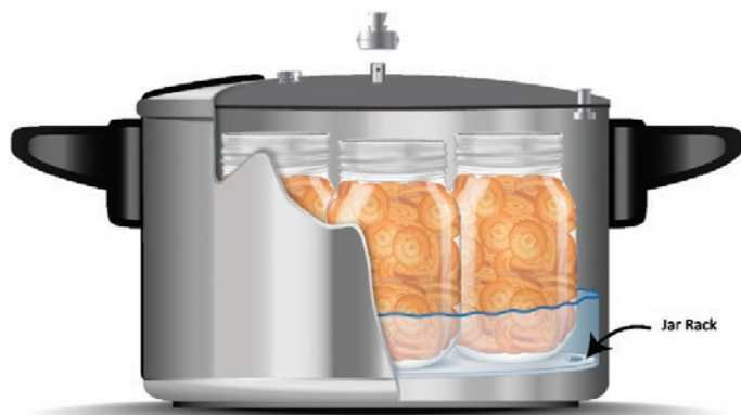
Figure 2. A 16-quart pressure canner allows for processing pint and quart jars in a single layer.
