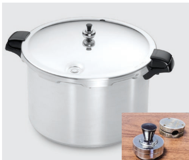
Figure 8. Weighted-gauge canners use a small round weight or disk on the canner vent pipe (inset) to control internal pressure.
