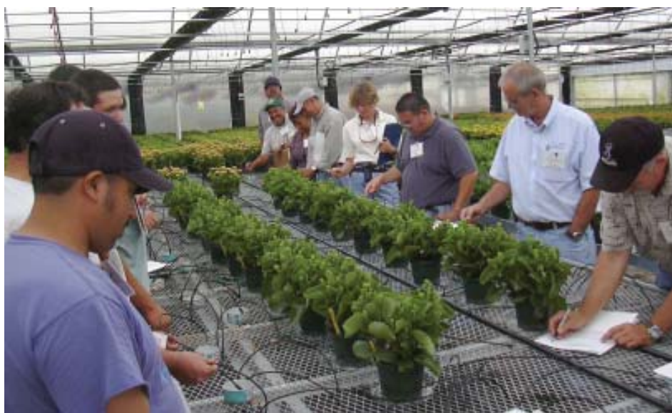
Workshop participants check irrigation uniformity using the can test.
