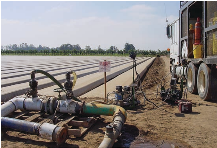
A company applies fumigant through drip irrigation in a strawberry field.
