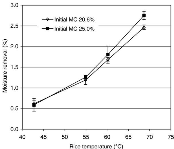
Fig. 2. Measured moisture removal (difference in moisture contents before and after heating) from rice samples with different initial MCs after heating to various temperatures.
