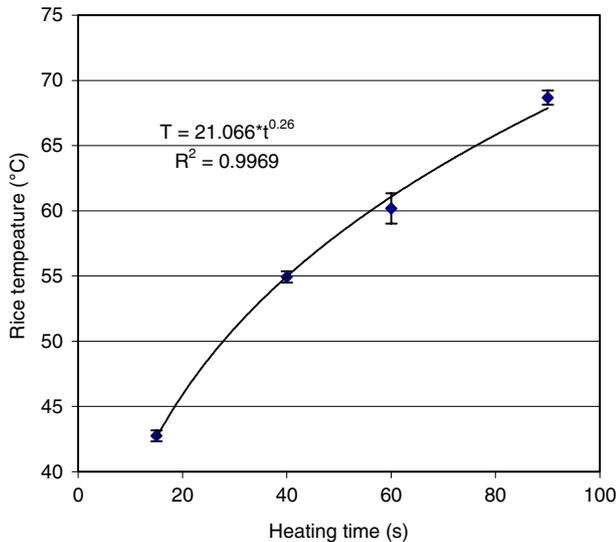
Fig. 1. Relationship between rice temperature and heating time.
