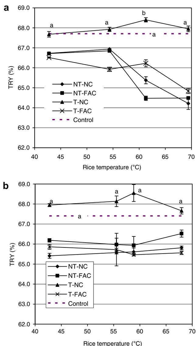
Fig. 5. Total rice yields (TRY) of rough rice with initial MCs of 20.6% (a) and 25.0% (b) under different drying treatments. (T – Tempering, NT – No tempering, NC – Natural cooling, FAC – Forced air cooling; Values with letter “a” were not significantly different from the control sample at  $p < 0.05$ .)
