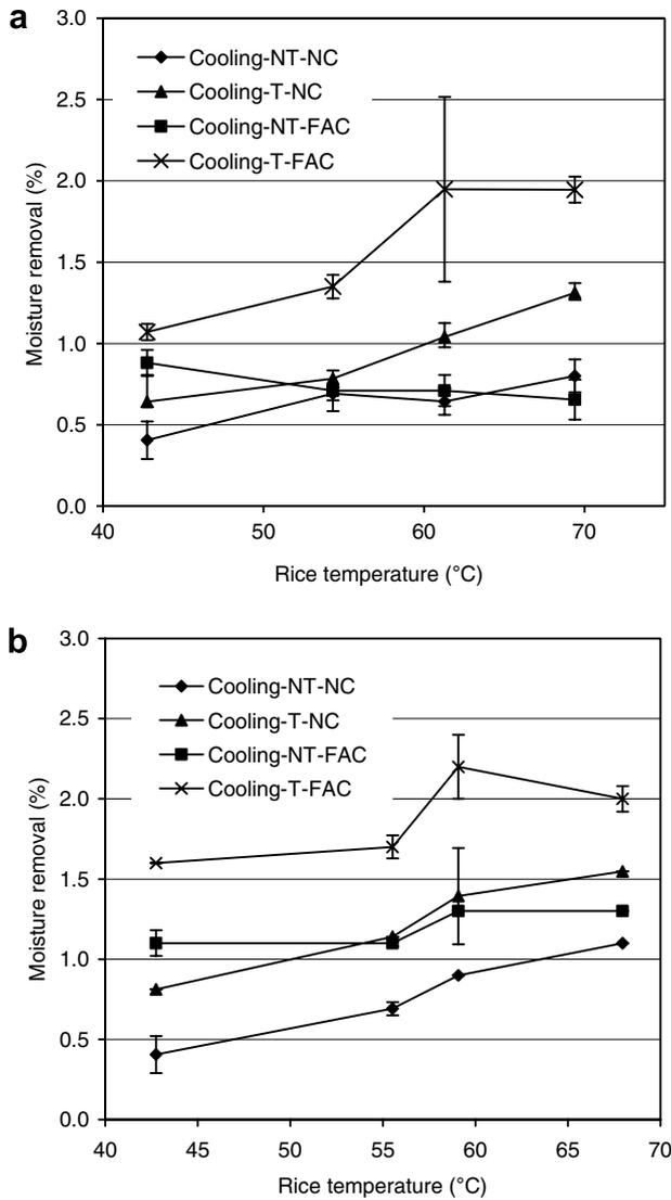
Fig. 3. Moisture removal under different cooling methods with and without tempering for rough rice with initial MC of 20.6% (a) and 25.0% (b). (T – Tempering, NT – No tempering, NC – Natural cooling, FAC – Forced air cooling.)
