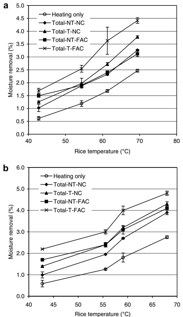
Fig. 4. Total moisture removal under different cooling methods with and without tempering for rough rice with initial MC of 20.6% (a) and 25.0% (b). (T – Tempering, NT – No tempering, NC – Natural cooling, FAC – Forced air cooling.)
