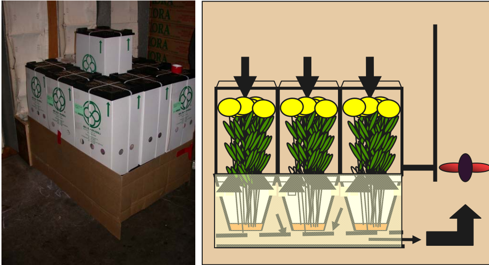
Pre-cooling Procona boxes on a conventional horizontal pre-cooler is achieved by directing the airflow down through the boxes using an adapter plenum, and a fiberboard or fabric sleeve around the base of the boxes.
