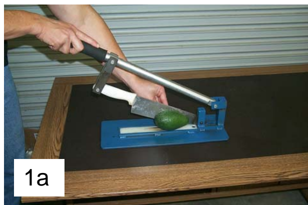
Figure 1. Overview of 1983 (Anon.) sampling protocol for an official dry matter determination; (a) Individual fruit is first longitudinally cut in half, (b) opposing eighths samples cut, (c) each eighth section peeled and seed material removed, (d) the ten opposing eighth sections from the 5-fruit composite sample, (e) composite sections placed in food processor, (f) ground tissue from the 5-fruit composite sample; a 5 gram sample is taken and dried in a microwave until constant weight is reached.
