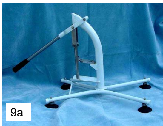
Figure 9. The tool designed for removing core samples from avocado; (a) an overview of the tool, (b) extraction of core from fruit, (c) the cored fruit and the extracted core sample.
