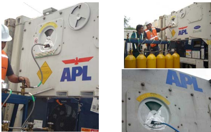
Required gas concentration is quickly achieved by N 2 gas flushing
