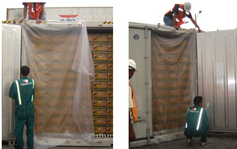
A Curtain is installed across the door to minimize leakage
