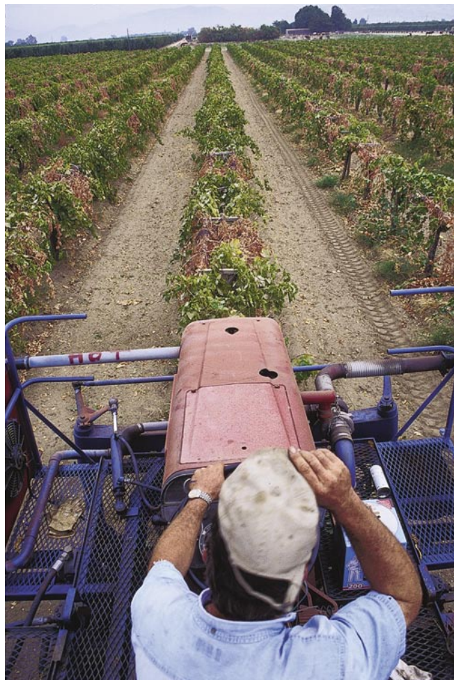
Above, dried-on-vine raisins can be mechanically harvested with a wine grape harvester. Below, hand-harvesting requires much higher costs for labor, paper tray disposal and preparation of clean middle rows.
