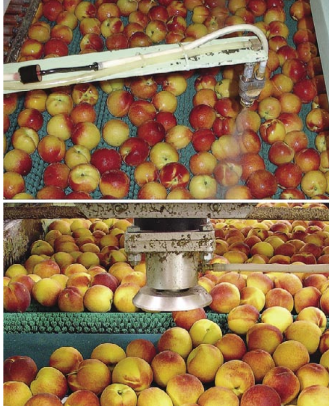
Without a postharvest fungicide treatment, fruit usually cannot be shipped to distant markets or displayed in the market at shelf temperatures without risking decay. Commercial, low-volume postharvest fungicide applicators include the "wigwag," top, and controlled droplet applicator, bottom, which are among the more popular methods because there is little to no fungicide runoff.
