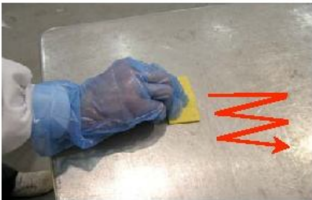
Figure 2. Hydrated sponge swabs are used to sample a process area surface.
