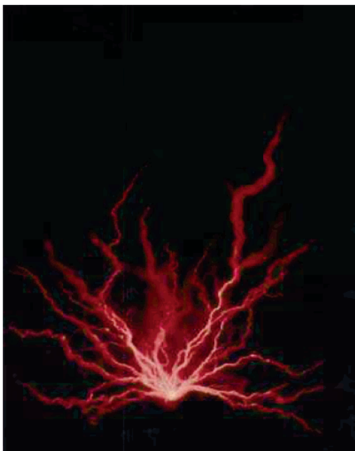
Figure 3. Photograph of streamers in liquid-phase pulsed corona discharge; time exposure is used to show the multiple discharge channels. (Reprinted from ref 410, with permission from the Japan Society of Applied Physics.)
