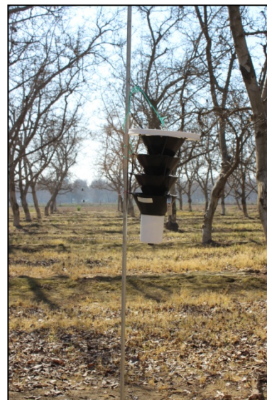
The latest design in walnut twig beetle traps employs a patent-pending pheromone to enhance beetle detection. Photo: E. Fichtner
