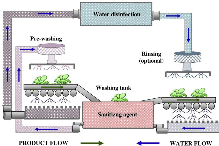
Fig. 2. Efficient water disinfection process with a re-circulation system proposed as an alternative for traditional fresh-cut washing.
