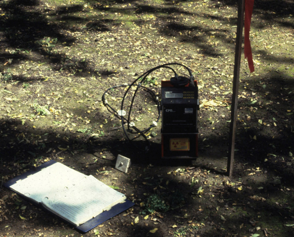
Campbell Pacific Neutron Probe at 8, 18, 30, 42 and 54 inch depths
