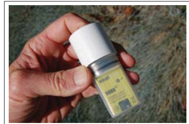
Figure 6. In order to assign each count to the corresponding plot or block when multiple areas are harvested in rapid sequence, it is necessary to record the precise time when the harvesting of one area ends and the next one begins. A separate datalogger with a push-button switch records this time precisely. Because this datalogger is programmed with the same computer as the harvest snips, all devices have the exact same clock setting.
