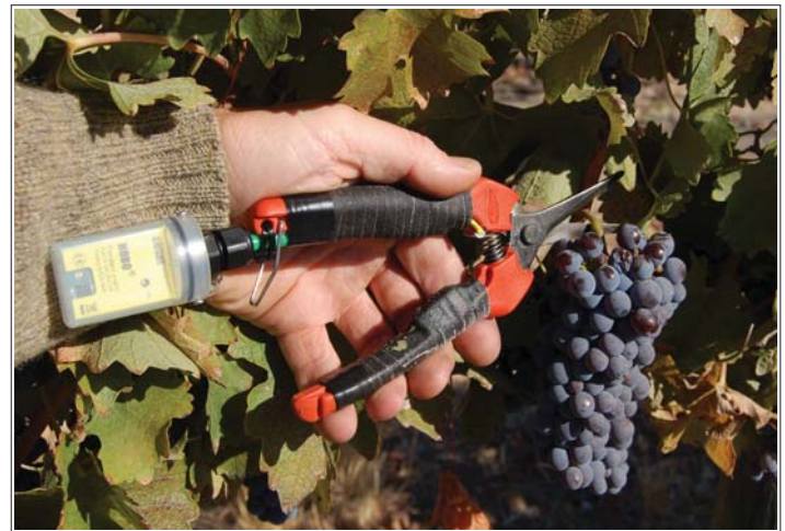
Figure 1. The datalogging harvest snips consist of a standard pair of Bahco® snips, outfitted with an Onset® Pendant™ Event datalogger and a magnetically-operated reed switch. The total materials cost per unit was about $110.
