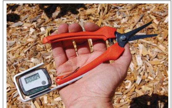
Figure 7. Another design uses an electronic counter with a numeric LCD screen; this device only tallies the total number of clusters harvested. The user resets the count to zero as needed with a button. The total materials cost per device is about $20.
