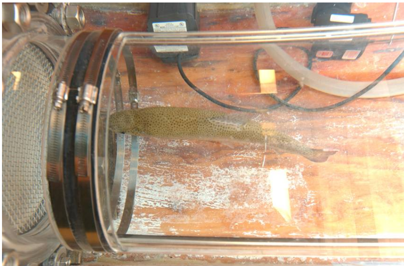
Figure 16. Researchers observing fish swimming during critical swimming velocity ( U_{crit} ) tests. The swim chamber was covered by curtains and the fish was observed on a live feed from a video camera. The receiver was placed on top of the video monitor so that the fish and EMG output could be viewed simultaneously.
