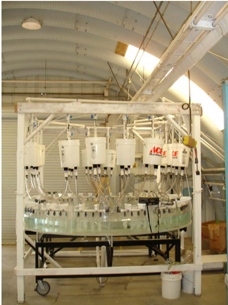
Figure 20. (a) Side view of temperature-preference apparatus and steel frame); (b) top view of same apparatus.
