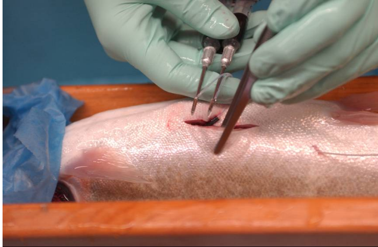
Figure 13. Electromyogram implant tool: gold-plated tag electrodes are placed into the grooves of two hypodermic needles and then forced out with 21-Ga steel rods attached to the syringe's rubber plunger.
