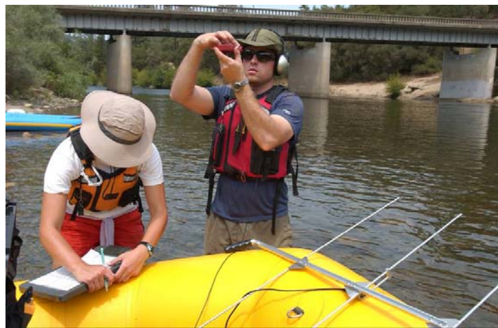
Figure 10. (a) Research team floating the river and listening as the receiver scans continuously for radio-tagged fish. (b) Researchers taking and recording bearings with a compass to triangulate a fish's location.
