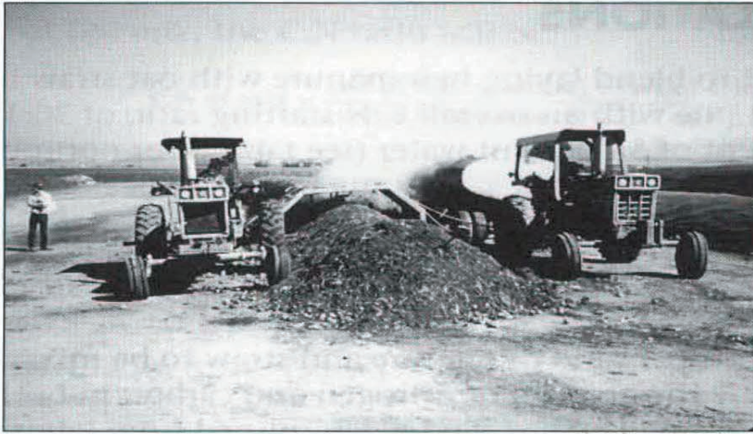
Figure 2. The PTO-powered compost turner (left) requires a tractor with a "creeper" gear that allows very slow travel. The tractor on the right is supplying water to replace moisture lost from evaporation during composting.
