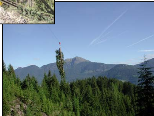
Top Left: skyline yarder on an excavator base. Credit: Jewell Manufacturing Bottom Right: Skyline yarding whole trees. Credit: Raffaele Spinelli
