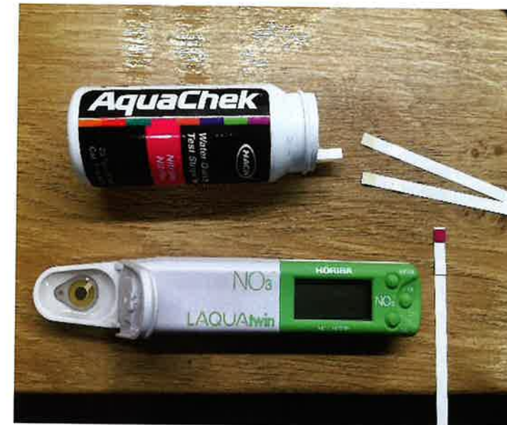
Figure 1. Example of colorimetric strips “Aquachek” (top) and a Horiba selective electrode meter (bottom). Note two unused colorimetric strips on the top right and one strip at the bottom right that was dipped into water and changed color according to the nitrate concentration.
