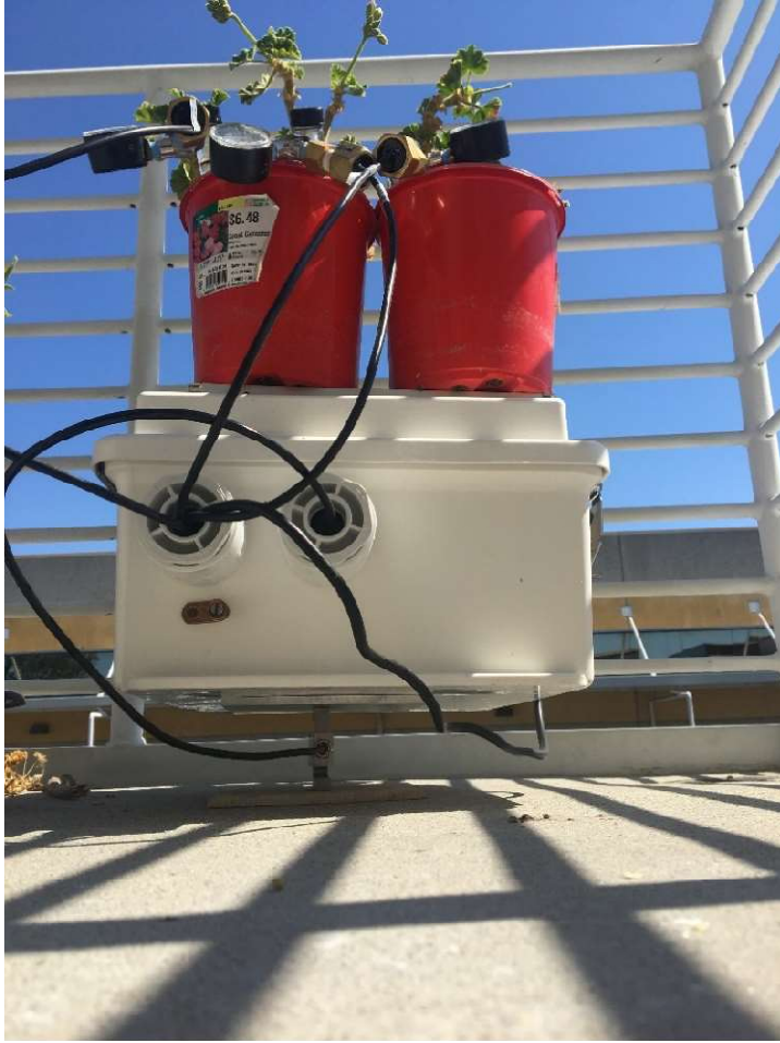
Figure 5. Geranium pots with tensiometers during the measurement. Note that we mounted the pots, datalogger enclosure and solar panel on the load cell to avoid that the cables affected the measured weight
