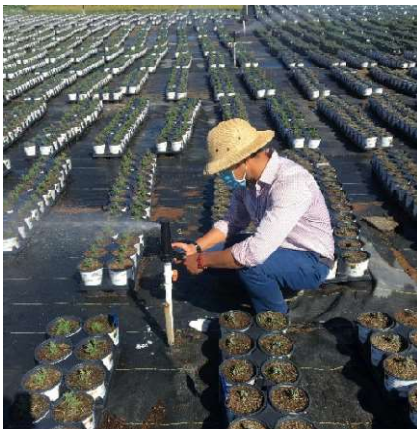
Figure 1. The Head Grower measuring pressure
