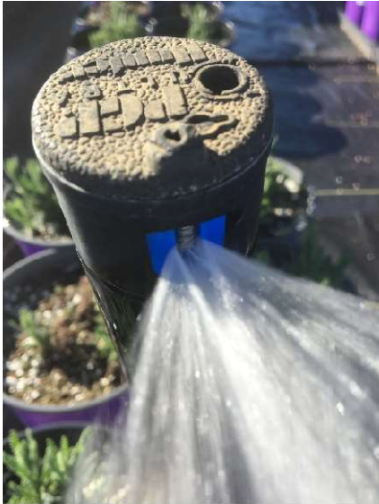
Figure 3. To reduce the radius, the nozzle screw was adjusted all the way in.
