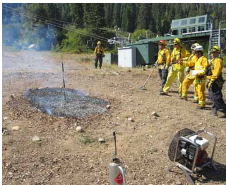
The study team partnered with local fire districts to measure burn characteristics of different mulches.
