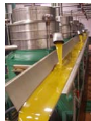
Vertical separators clarifying the oil
