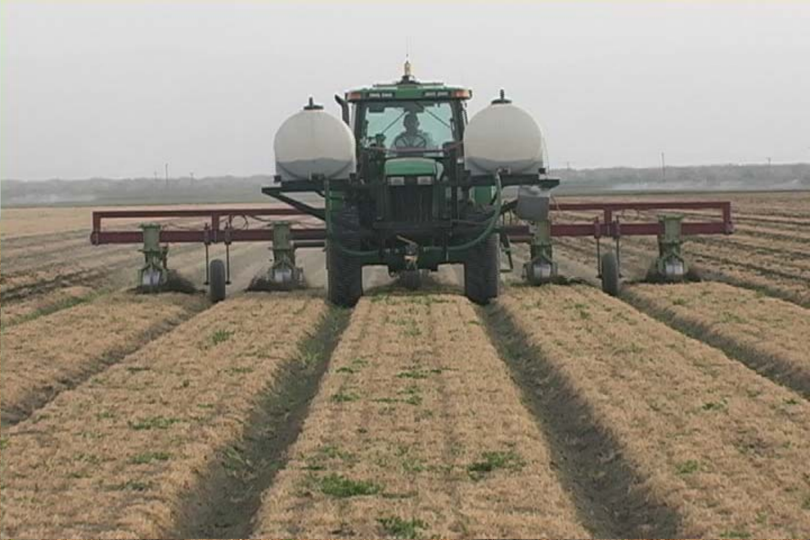
Ground-driven strip-tiller ahead of transplanting Firebaugh, CA 2009
