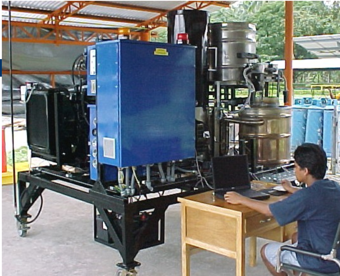
Community Power Corp Gasifier - 12.5 KW, Philippines
