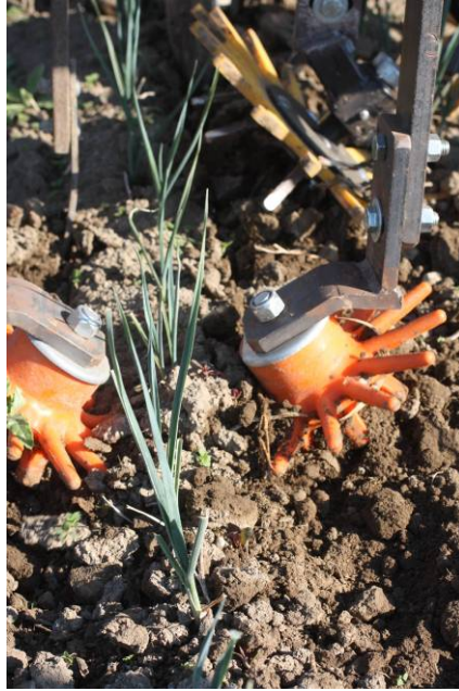
Figure 2. 9.5 inch finger weeders rotate and up root small weeds. They can be more or less aggressive to the weeds and crop by adjusting the distance between them.
