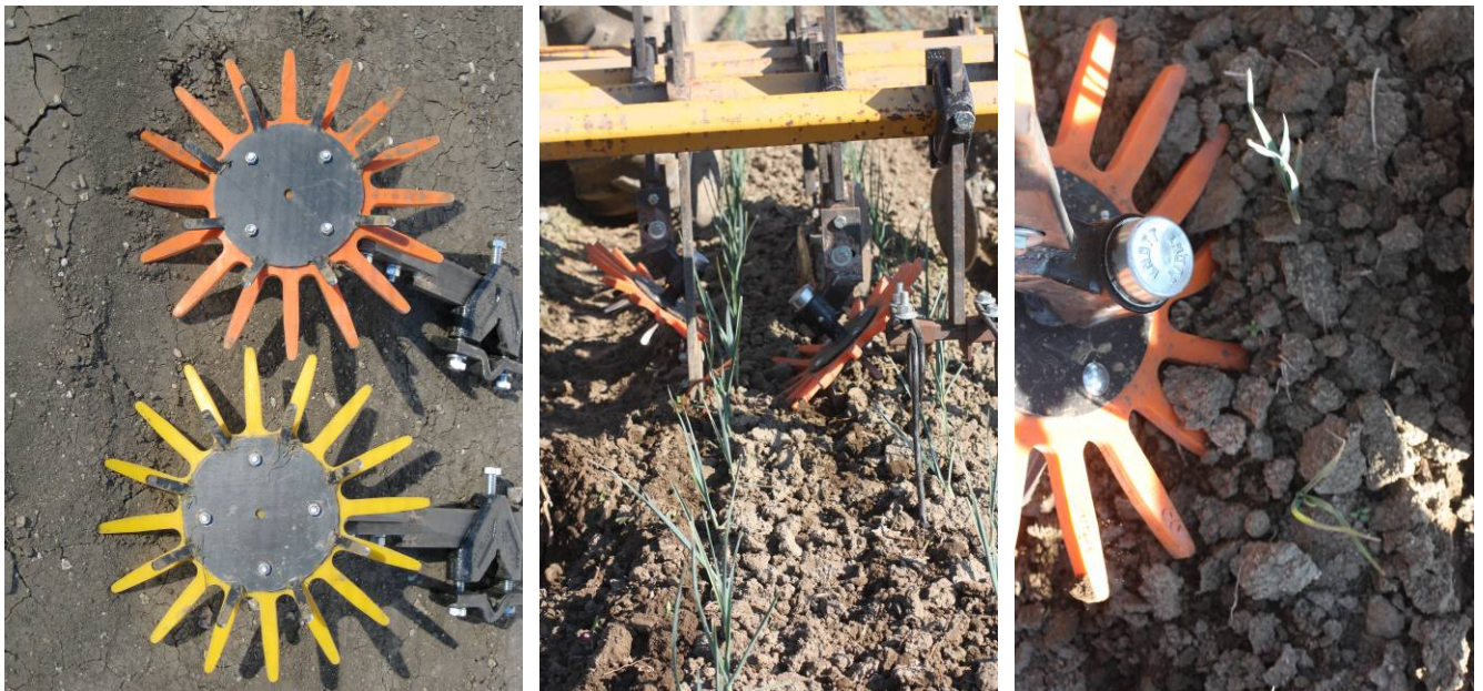
Figure 1. 14.5 inch in diameter finger weeders. The orange are softer and the yellow are harder which allows you to select their aggressiveness. The fingers are ground driven and spin faster than the ground speed, thereby flipping young weeds out of the ground.
