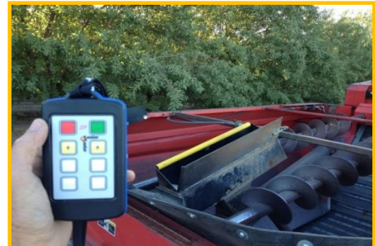
Wireless controller for hydraulically operated auto sampler
