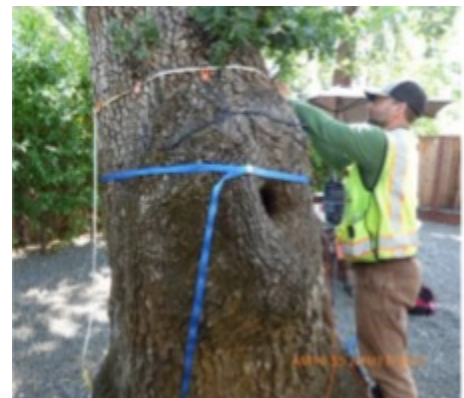
An arborist using a tomograph, a tool used to detect decay and assess the interior health of a tree.
