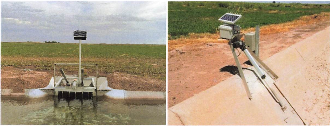
Fig. 1. Two automated surface irrigation fields in Imperial Valley. Two different automated gates are demonstrated in klein grass and alfalfa fields.
