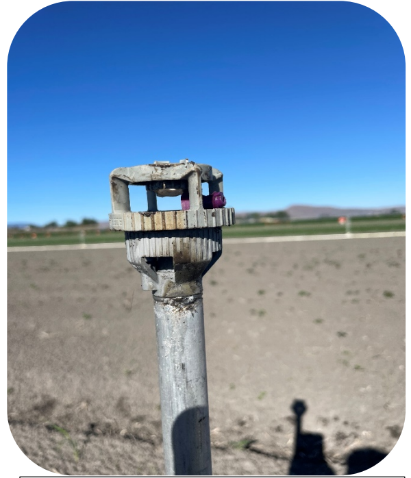
Melted Sprinkler from Lightning Strike
