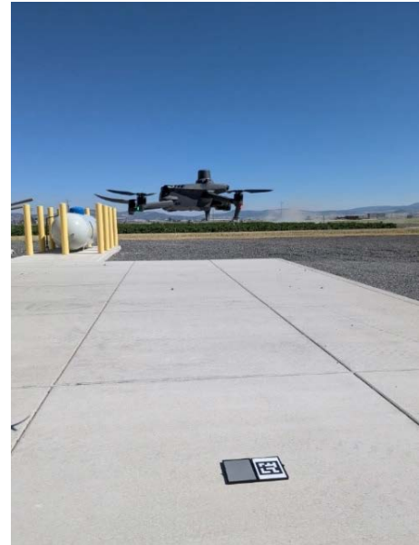
Figure 1: Capturing a drone image from a calibration panel at IREC.
