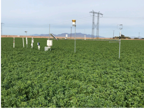
Fig. 8 A fully automated surface renewal and eddy covariance evapotranspiration (ET) tower in a commercial alfalfa field in Palo Verde, CA.
